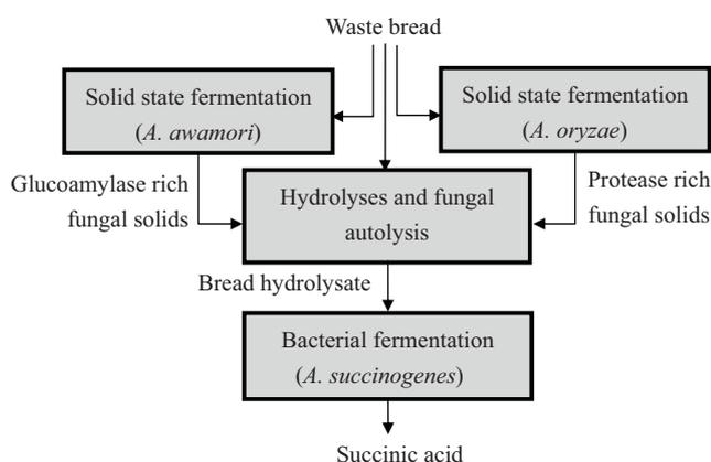
**Fig. 1.** Process flow diagram of the proposed waste bread biorefinery concept for succinic acid production. The biorefinery consists of three steps: (1) *A. awamori* and *A. oryzae* SSF were carried out on waste bread to obtain glucoamylase and protease-rich fungal solids. (2) The solids were added to a waste bread suspension to produce a nutrient-rich hydrolysate. (3) *A. succinogenes* fermentation using the waste bread hydrolysate for SA production.
